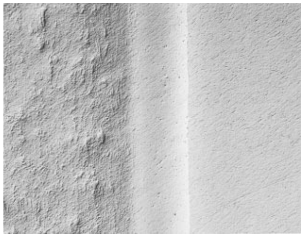
Figure 5. 200 \times microscopic image of sample a . The bulk of the PMR-15 sample is shown on the left side adjacent to the 0.2 mm smooth surface layer in the mid-vertical section. The remainder of the smooth region to the right of the surface layer is the epoxy resin used to mount the sample. The surface layer is found to be richer in oxygen than the sample bulk.
